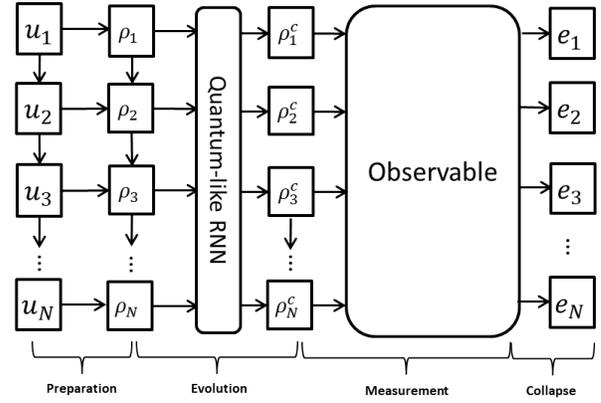
Figure 2: Diagram of the proposed network. Each utterance  $u_j$  is represented by density matrix  $\rho_j$ . The evolution step is a Quantum-like RNN. Post-evolution states  $\{\rho_j^c\}$  are fed into the measurement controlled by observable  $O$ . The emotions with the largest likelihood  $\{e_j\}$  are produced.
