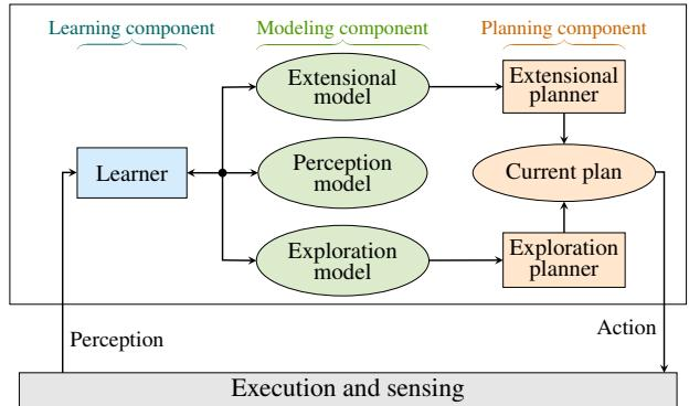
Figure 1: PAL architecture. The square boxes represent modules; the circle ones represent data.
