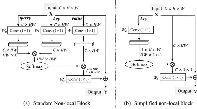
Figure 3: The architectures of a standard non-local block and a simplified non-local block. “ $\otimes$ ” denotes matrix multiplication and “ $\oplus$ ” denotes broadcast element-wise addition.
