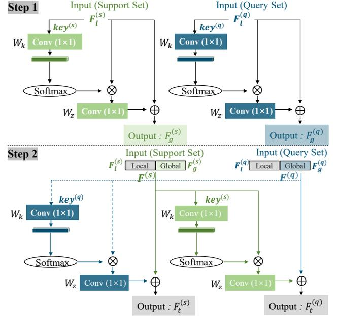
Figure 4: The architecture of Cross Non-Local Neural Network. At step one, it captures the long-range dependency for the samples in support and query set, respectively. At step two, it extracts the task-specific features.
