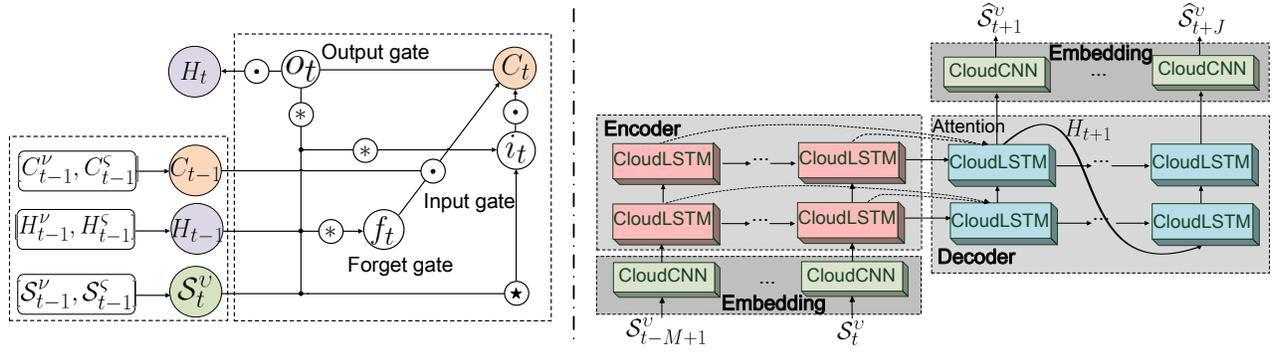
Figure 3: The inner structure of the CloudLSTM cell (left) and the overall Seq2seq CloudLSTM architecture (right). We denote by  $(\cdot)^v$  and  $(\cdot)^s$  the value and coordinate features of each input, while these features are unified for gates.
