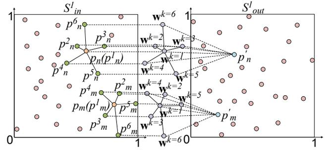
Figure 2: DConv operation with a single input channel and  $\mathcal{K} = 6$  neighbors. For every  $p \in \mathcal{S}_{\text{in}}^i$ , DConv weights its  $\mathcal{K}$  neighboring set  $\mathcal{Q}_n^{\mathcal{K}} = \{p_n^1, \dots, p_n^{\mathcal{K}}\}$  to produce values and coordinate features for  $p'_n \in \mathcal{S}_{\text{out}}^j$ . Here, each  $w^k$  is a set of weights  $w$  with index  $k$  (*i.e.*,  $k$ -th nearest neighbor) in Eq. 2, shared across different  $p$ .
