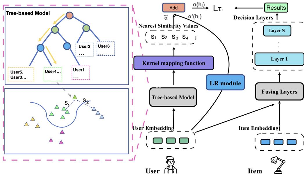
Figure 2: The network structure of the tree-based PAML. The right part is the network for inner update while the left part is the tree-based module. Specifically, *Fusing Layer* indicates the concatenation of user and item embeddings, *Add* is an adding function:  $\alpha'(h_i) + \tilde{\alpha}$ . *Layer1, \dots, N* means fully connected layers and  $S_1, \dots, S_4$  are similarity values.
