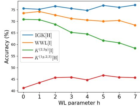
Figure 2: Different outcomes of  $h$  parameter when employing WL in Hilbert space [H] and input space [I] in four methods. The experiment was done on the ENZYMES dataset.
