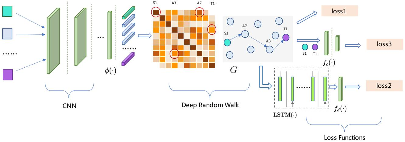
Figure 2: The architecture of the DERWENT model can be divided into three parts: (1) Images features are extracted by a pre-trained deep convolution neural network (CNN) followed by the feature extraction network  $\phi(\cdot)$ . (2) According to the hidden feature representation generated in the previous step, we construct a graph  $G$  on each mini-batch data points and adopt the random walk to generate transfer paths. (3) Three losses are calculated based on the sampled sequences.
