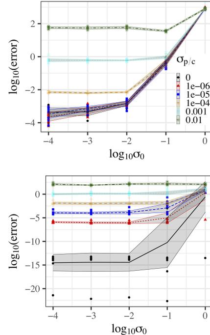
Figure 3: OTTER recovery error using (top) gradient descent and (bottom) spectral decomposition for artificial networks of size  $n_p = 100$ ,  $n_c = 200$  and Gaussian noise with variance  $\sigma_{p/c}^2$  for  $P$  and  $C$  and  $\sigma_0^2$  for  $W_0$ . Shaded regions correspond to the 0.95 confidence interval and lines to the average over 10 repetitions. The legend applies to both figures.
