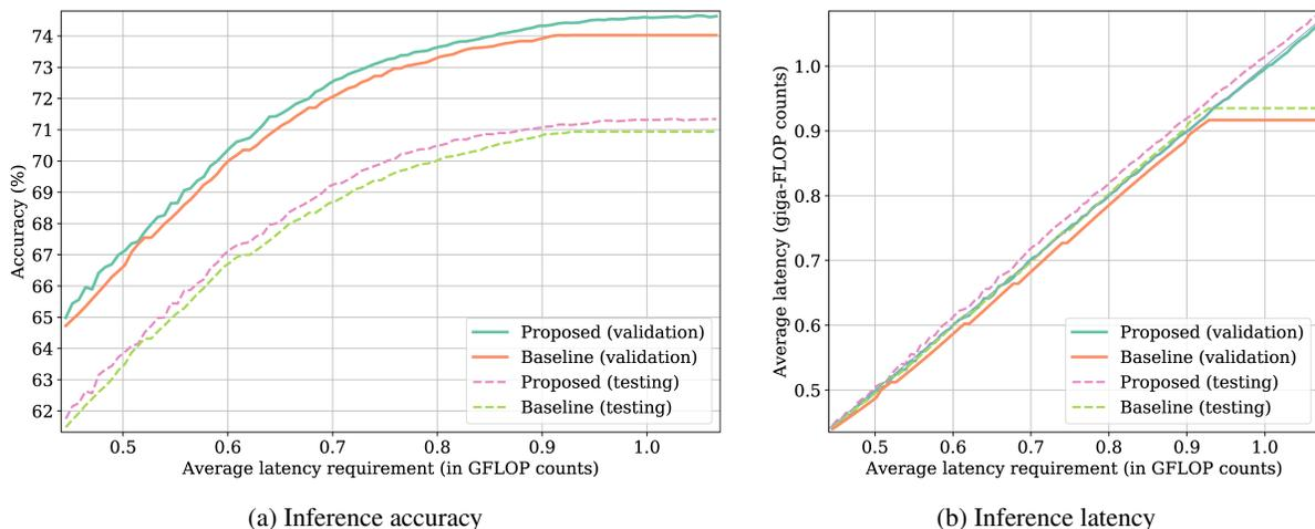
Figure 4: Experimental results on MSDNet over ImageNet.
