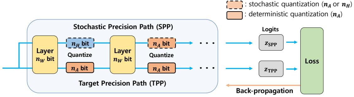
Figure 1: Structure of the proposed SPEQ training scheme for QDNNs. The QDNNs are trained for the target precision  $n_A$  through the ‘target precision path’. The ‘stochastic precision path’ produces the teacher logits,  $\mathbf{z}_{\text{SPP}}$  using the same model but with randomly assigned quantization precision for activation at every iteration. Note that the weights in the model are quantized to  $n_W$  bits.
