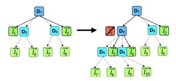
Figure 3: The dynamic growth process with a deeper PRO-LONET shown in paler colors and dashed lines. When  $H(\vec{l_3}) + H(\vec{l_4}) < H(\vec{l_1})$ , the agent replaces  $\vec{l_1}$  with  $D_2$ ,  $\vec{l_3}$ , and  $\vec{l_4}$  and adds a new level to the deeper actor.
