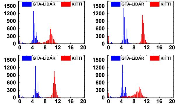
Figure 4: Pixel-wise feature distribution at four sampled locations on the  $x$  coordinate channel of 5,000 projected LiDAR images from GTA-LiDAR (Wu et al. 2019) and KITTI (Geiger, Lenz, and Urtasun 2012; Wu et al. 2018a). The ordinate represents the number of images, while the abscissa represents the detailed  $x$  values.
