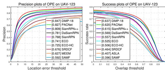
Figure 5: Precision and success plots of OPE on UAV-123.
