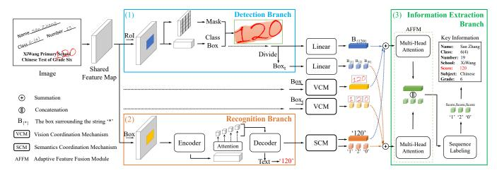
Figure 3. The overall framework of VIES. It consists of a shared backbone network and three specific branches: (1) text detection, (2) text recognition and (3) information extraction.  $Box_t$  denotes boxes of single tokens which divided from the box of entire text segment Box.
