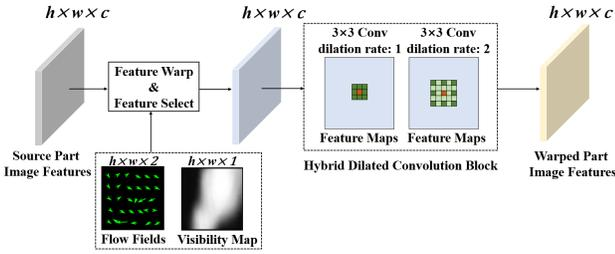
Figure 3: The local warping module. It warps the source features encoded from the corresponding part images to align them with the target pose while capturing the short-range semantic correlations of local neighbors within the parts.
