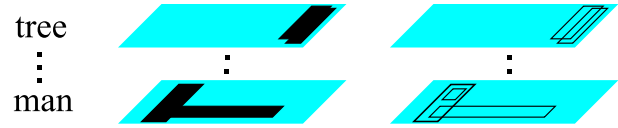
Figure 4: Blue indicates 0 and black indicates 1. (Left) The per-class mask constructed from the layout by many previous methods makes it impossible to distinguish unique object instances in several cases. (Right) Our mask consists of instance boundaries making it easier for the model to distinguish unique object instances using no extra information than already contained in the layout.
