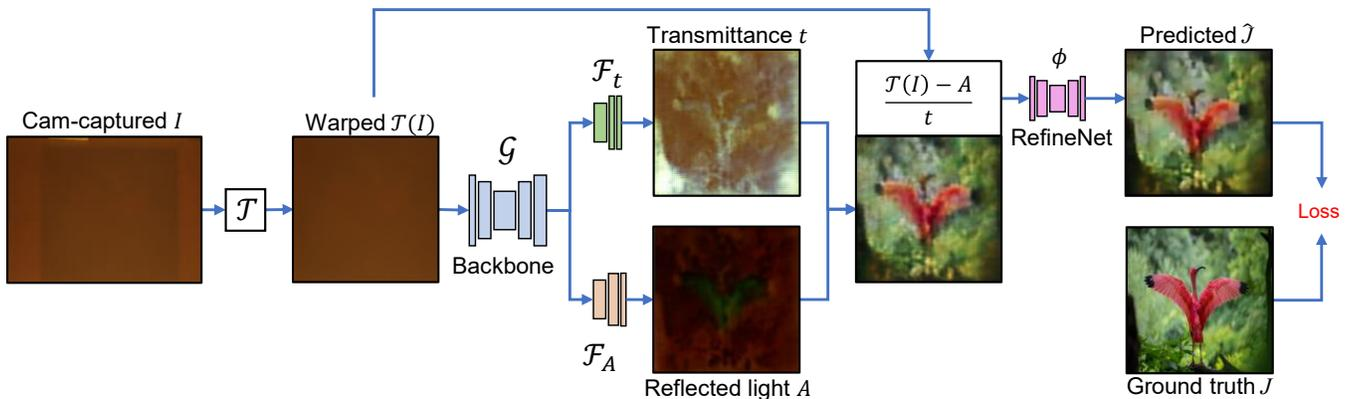
Figure 2: Network architecture of our Neural-STE. It consists of three modules: WarpingNet  $\mathcal{T}$ , DehazingNet ( $\mathcal{G}$ ,  $\mathcal{F}_A$ ,  $\mathcal{F}_t$ ) and RefineNet  $\phi$ . These modules together with the losses allow us to utilize our image formation model to effectively model privacy attacks on physical mail problem.
