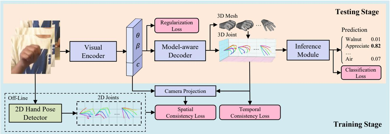
Figure 2: Overview of our proposed framework. The framework consists of a visual encoder, a hand-model-aware decoder and an inference module. Jointly with the video-level supervision, we further constrain the spatial and temporal consistency of intermediate 3D pose representations for further performance improvement. The modules utilized in training and testing stages are highlighted in light blue and orange, respectively.
