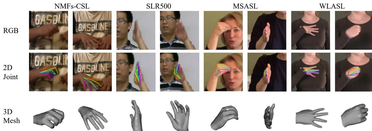
Figure 3: Visualization of the intermediate mesh representation. From the first to the third row, we present the RGB hand, 2D joint detected by OpenPose and the 3D mesh generated by our method. We visualize one sample in the test set for each benchmark dataset, including NMFs-CSL, SLR500, MSASL and WLASL. For each sample, we visualize two key frames.
