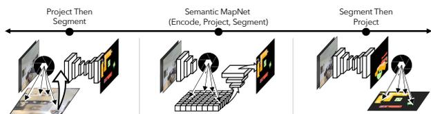
Figure 2: A spectrum of approaches to top-down semantic segmentation: (Right) perform egocentric semantic segmentation and project *labels*; (Left) Construct an overhead imagery (project *pixels*) and perform semantic segmentation; (Middle) SMNet: encode pixels, project *features*, decode labels.
