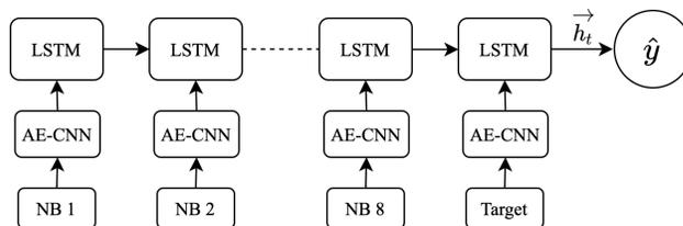
Figure 3: The relational-LSTM (R-LSTM) architecture. The images of the eight neighbors and the target cell, as shown in Figure 2, is treated as sequence of inputs. The AE-CNN is a convolutional encoder, which is initialized using the weights of an auto-encoder trained on unlabeled data  $\mathbf{U}$  using unsupervised learning. The target of the R-LSTM is the label of the target cell.
