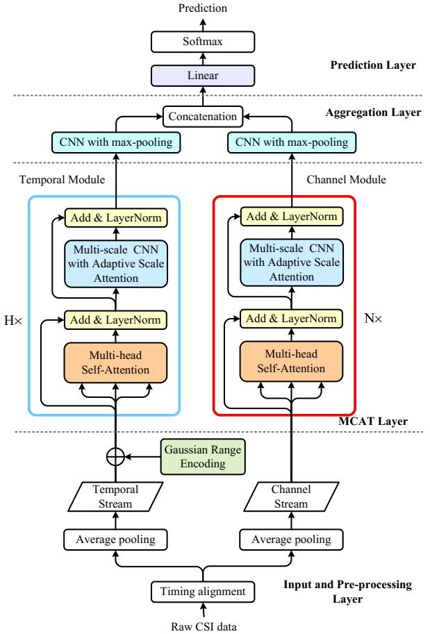
Figure 2: Architecture of THAT Model.
