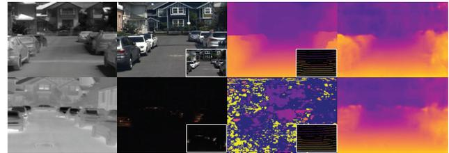
Figure 1: The result of an accurate depth estimation using a *Multispectral Transfer Network* (MTN) in both day (top) and night (bottom) conditions. From left to right: input thermal images, RGB stereo pairs, depths from RGB stereo/Velodyne HDL-32E, and our results. The proposed method can predict high-quality pixel-wise depths at night compared to the depths from the RGB stereo/Velodyne.
