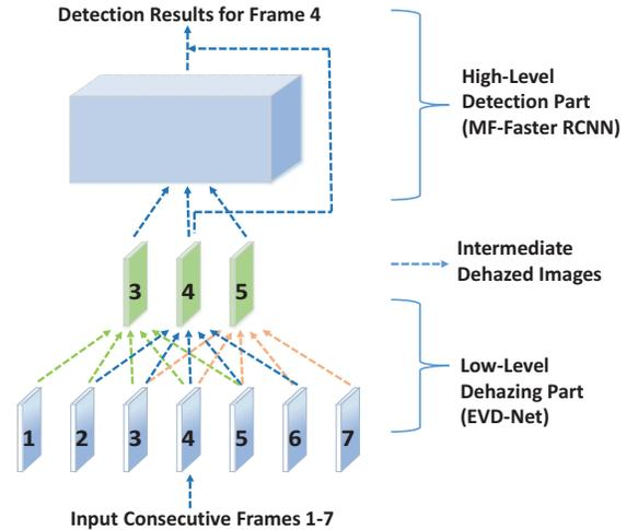
Figure 3: EVDD-Net for united video dehazing and detection, with a tree-like deep architecture. Note that the entire pipeline will be jointly optimized for training.
