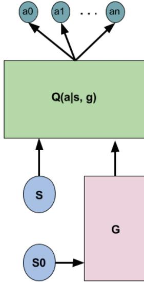
Figure 1: The goal generator generates a goal, and the Q function approximates action values for all actions conditioned on the current state and the given goal
