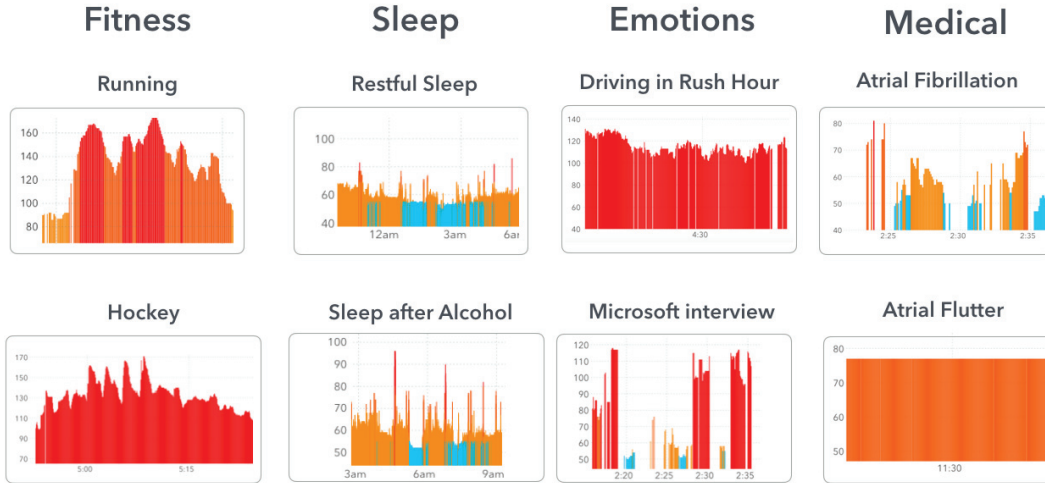
Figure 1: Examples of wearable heart rate data showing different physiological states: exercise, sleeping, stress, and medical conditions.
