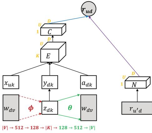
Figure 3: Neural network view of NIPEN-Tensor. The contents part is connected with the blue line (with content scaling parameter  $\alpha_u$ ), and the network part is connected with the purple line (with the network scaling parameter  $\beta_u$ ).
