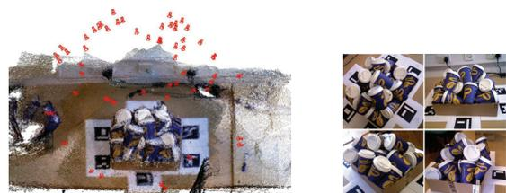
Figure 4: (left) Accumulated view and camera pose of different view of a pile of coffee cup scenario; (right) images from four different views.
