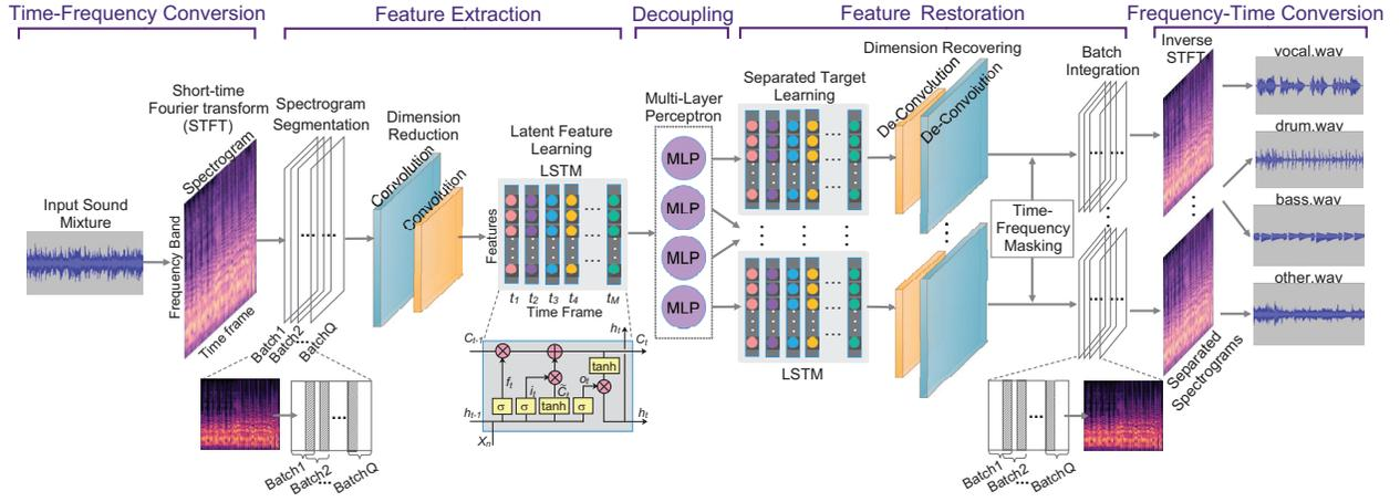
Figure 2: Illustration of architecture of Deep Representation-Decoupling Neural Networks (DRDNN).
