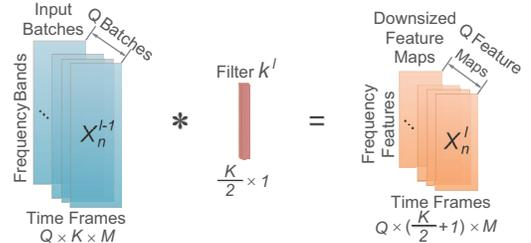
Figure 3: Convolution for frequency-dimension reduction.
