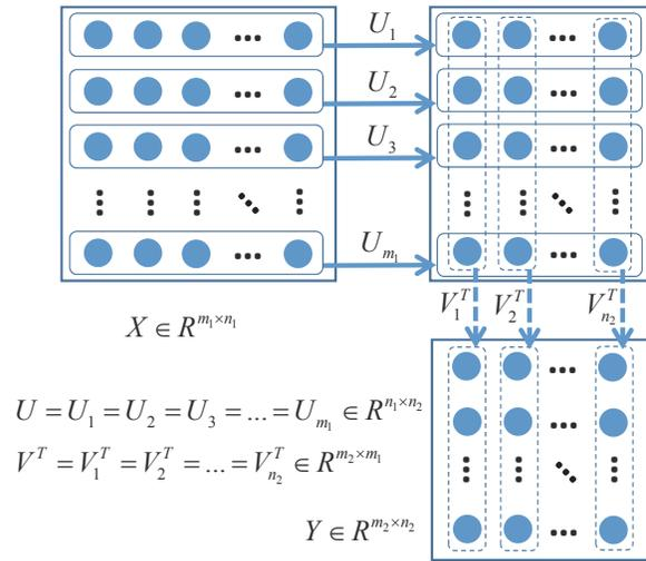
Figure 2: The illustration of the 2D fully connected layer. Neurons in the rectangles connecting to an arrow are fully connected each other. The solid line represents the first step, and the dotted line represents the second step.
