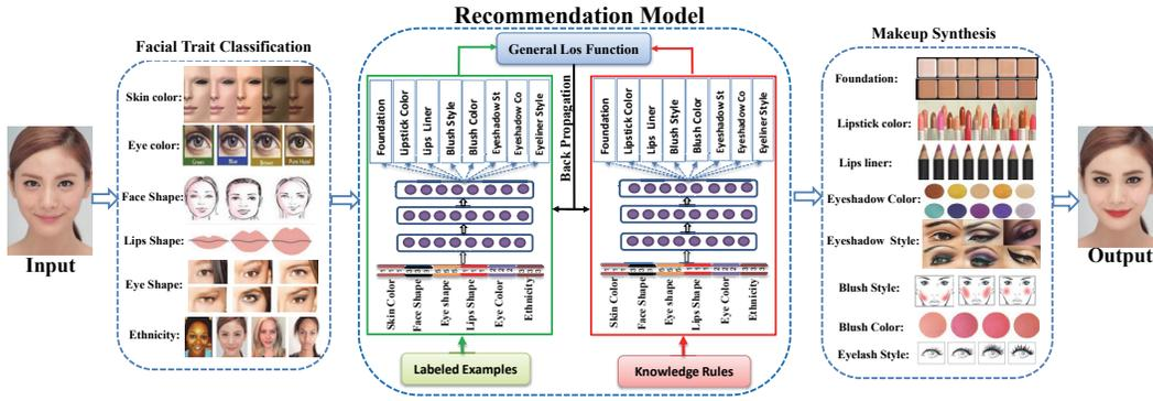
Figure 1: Overview of our proposed framework. It shows the automatic classification of the facial attributes, Examples-Rules deep learning recommendation system and the synthesis results of the recommended makeup .
