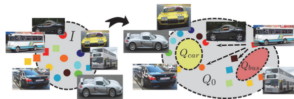
Figure 1: We learn a global metric Q_0 to discriminate classes and preserve global view-specific appearance, as well as class-specific pose estimation metrics Q_{car} and Q_{bus} . This joint learning allows to predict the pose for instances of novel object classes. For example, we can estimate the pose of the class bus by utilizing the view labels for class car , which is its neighbor in the class space.
