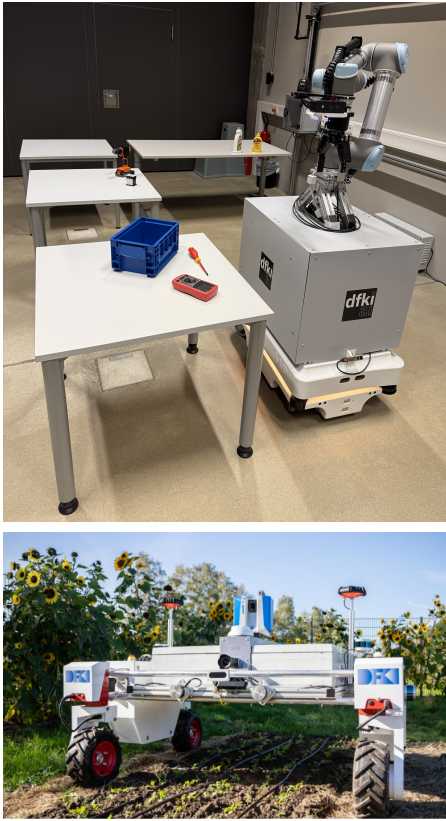
Figure 1: Robotic platforms used in our experiments (see Section 6): the Mobipick mobile manipulator (top), operating in the object collection scenario, and the Valdemar robot (bottom), operating in an agricultural environment.
