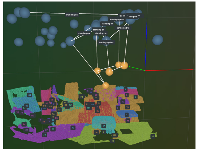
Figure 4: Visualization of local scene graph (yellow) and global scene graph (blue) with inter- and intra-layer edges with a mapped scene from the 3RScan dataset. Predicted edges are integrated into the global graph using ground truth annotations from Wald et al. (2020).
