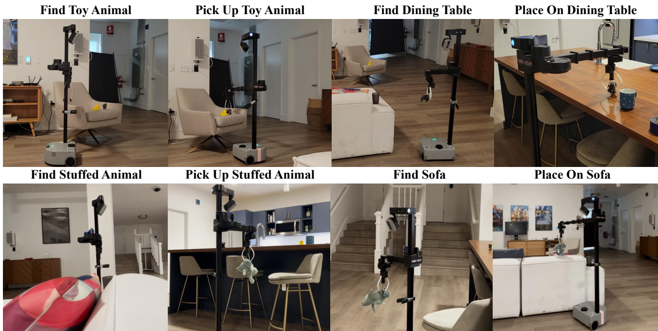
Figure 3: The HomeRobot stack being used to perform the Open Vocabulary Mobile Manipulation task in a held-out, real-world test environment. The test environment is a mock apartment which will be used for multiple versions of the benchmark, including for the HomeRobot Neurips 2023 competition (Yenamandra et al. 2023a). This allows us to perform both simulated and real-world benchmarking of new methods, and will help center the community around a broadly-available, low-cost platform with growing capabilities.
