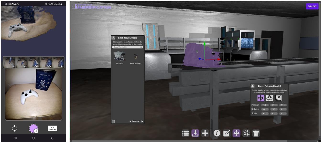
Figure 1: The prototype of the capture client (left) showing imagery being captured, and a 3D reconstruction of using the captured imagery. And, a prototype for the editing client (right) showing how 3D reconstruction models can be manipulated and used to populate virtual environments.
