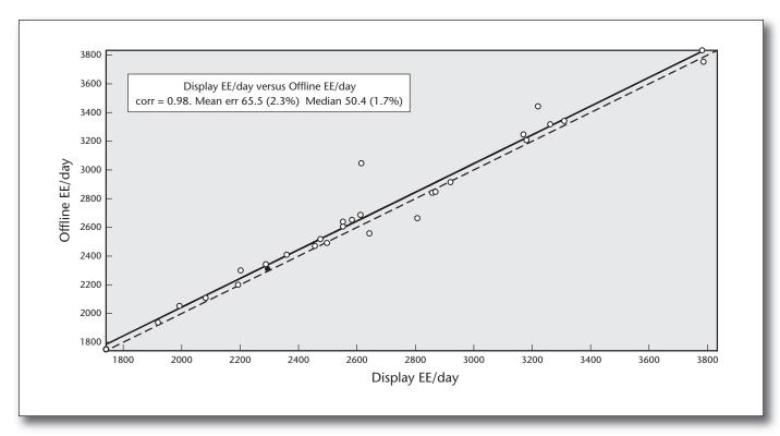
Figure 5. Comparison of Display EE Versus Offline EE. The correlation is 0.98 and the mean difference is 2.3 percent.
