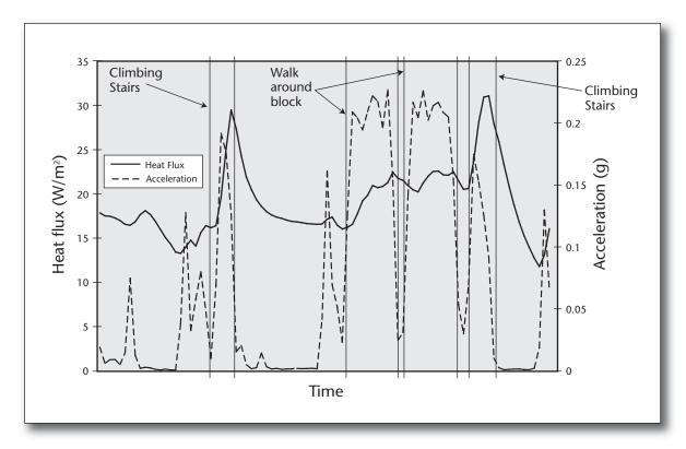
Figure 2. A Sample of Armband Signals during Various Activities. Multiple sensors allow better activity classification.
