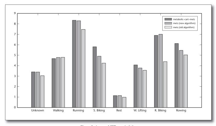
Figure 3. Average METs per Activity. Ground truth computed from metabolic carts, for current algorithm and new release candidate.
