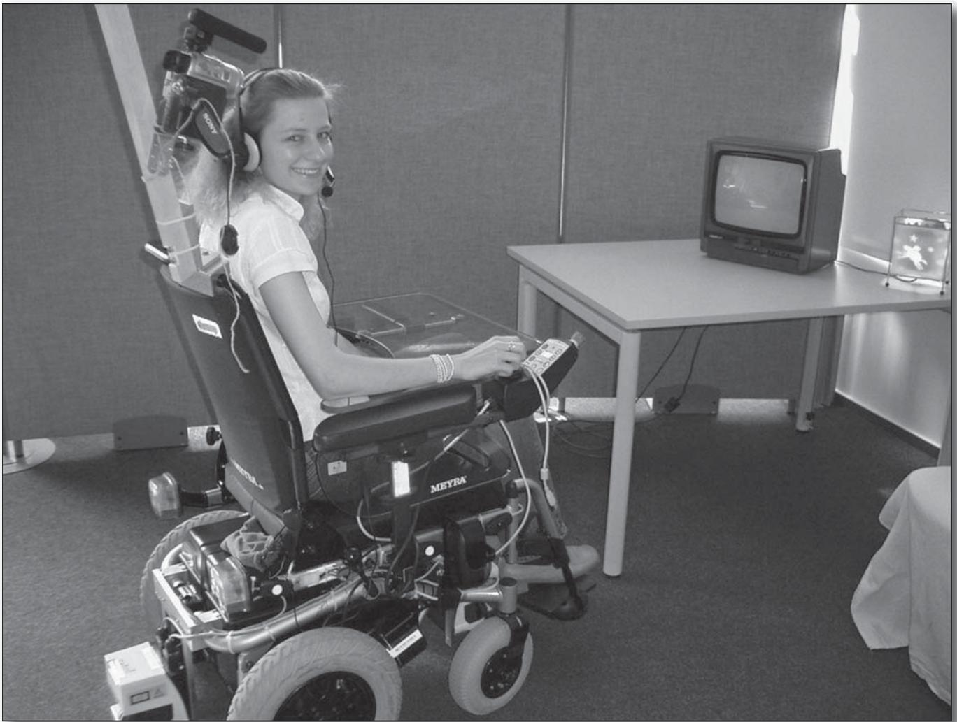
Figure 1. The Robotic Wheelchair "Rolland."
