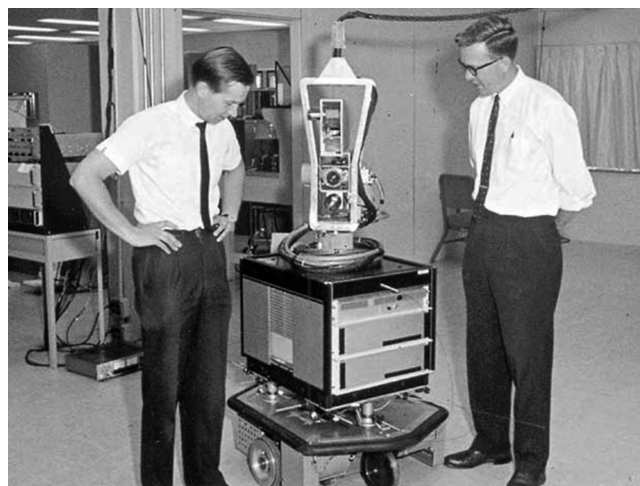
FIGURE 3 Shakey the robot implemented the STRIPS planning algorithm (Fikes and Nilsson 1971)
