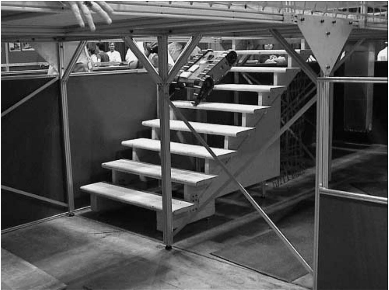
*Figure 3. University of South Florida Robot Descending Steps in the Medium-Difficulty Section of the Urban-Search-and-Rescue Arena (courtesy of William Adams).*
