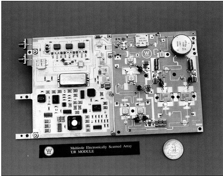
Figure 8. The Same Basic Approach (and Even Some of the Same Code!) That We Used for Planning Declarer Play in *BRIDGE BARON* Is Also Used in a Program That Plans How to Manufacture Microwave Transmit-Receive Modules (MWMs), Such as the One Shown Here.
