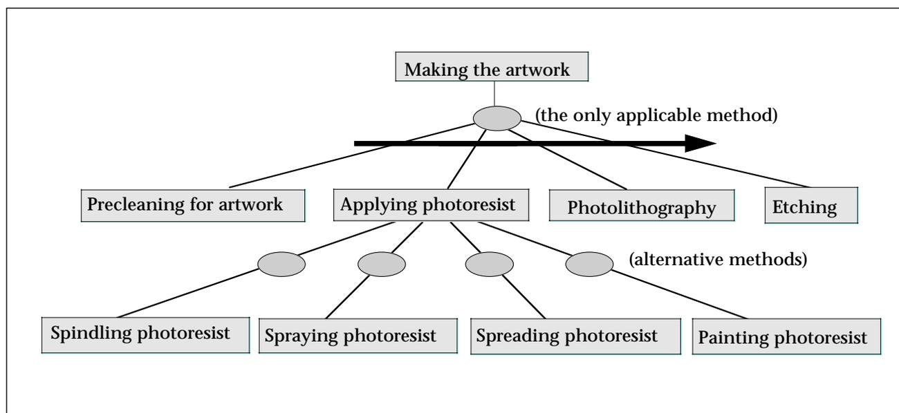
Figure 9. A Portion of a Task Network Containing Operations Used in Manufacturing Microwave Transmit-Receive Modules (MWMs).
